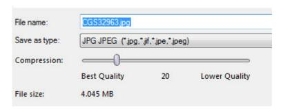
The scale ranges from 1 to 99. In the example above, it is set to 20.
