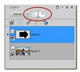
7- Adjust the placement of the shape as you want. You can also resize it, or rotate it. Since it is a vector shape, the edges will stay well-defined.
