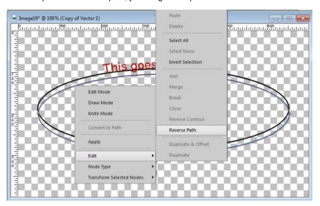
Once you have a REAL path, that is now reversed, whenever you type, the text will go in the counterclockwise direction. Of course, that means that you will want the text on the bottom part of the ellipse, or it will become upside down when the text is on top.
