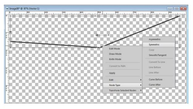
Reduce the length of the arrow on the end nodes to a minimum, and for the middle one, adjust it so you get a nice, and smooth curve, from left to right.
